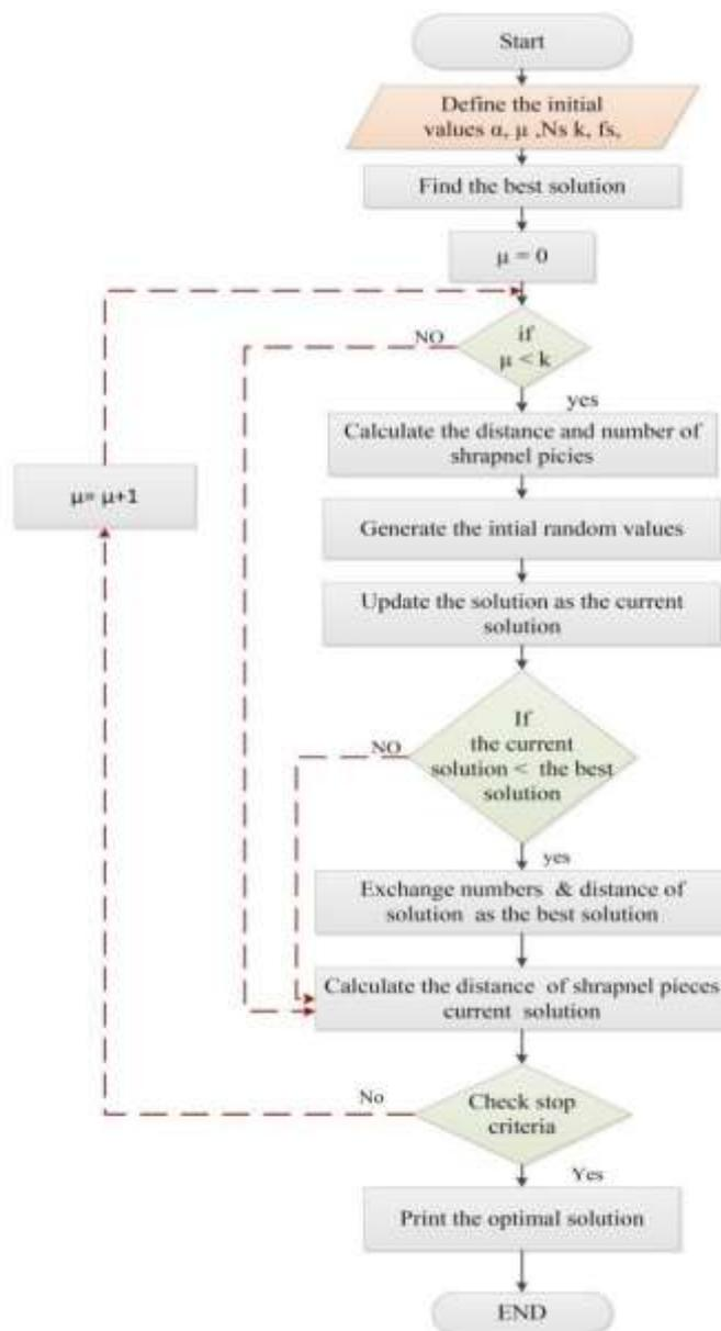
Figure 5. Flow chart of mine blast algorithm
