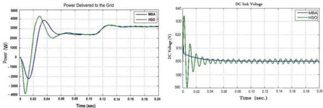
**Figure 9.** The power delivered to grid for the two techniques **Figure 10.** The DC link voltage for the two techniques
